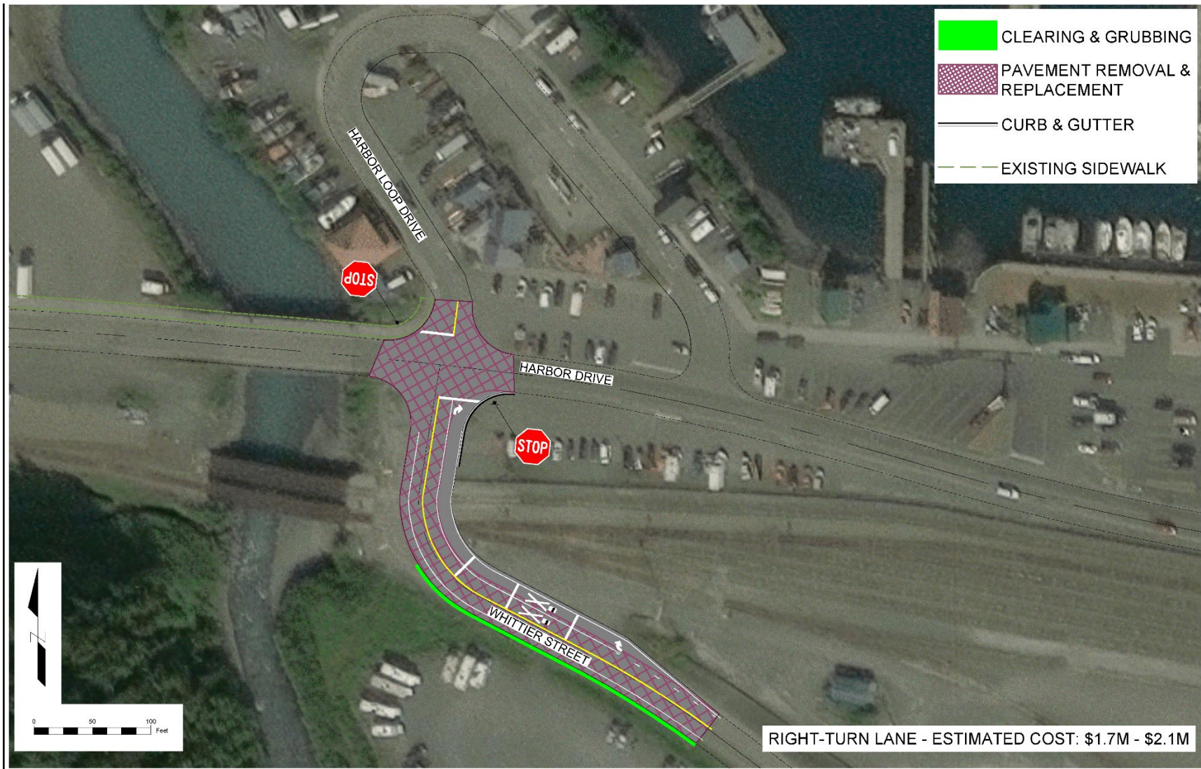
Figure 17: Conceptual Design - Whittier Street Turning Movements Variation B
